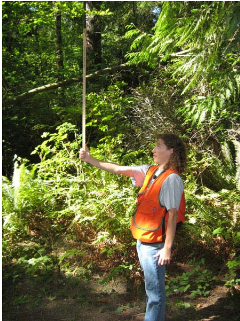
Figure 6-6: When measuring height with a woodland stick, hold the stick 25 inches from your eye and keep the stick vertically straight.
