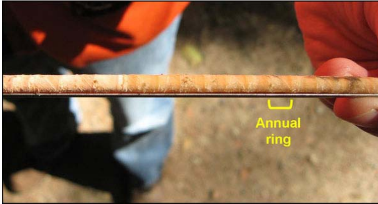
Figure 6-9: An increment borer allows you to extract a small core sample from the stem of the tree with which you can determine age by counting the annual rings.
