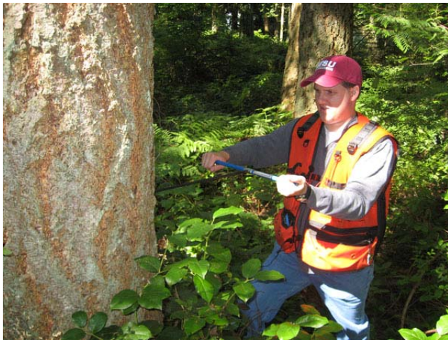
Figure 6-12: When using an increment borer, drill in straight toward the center of the tree at breast height.
