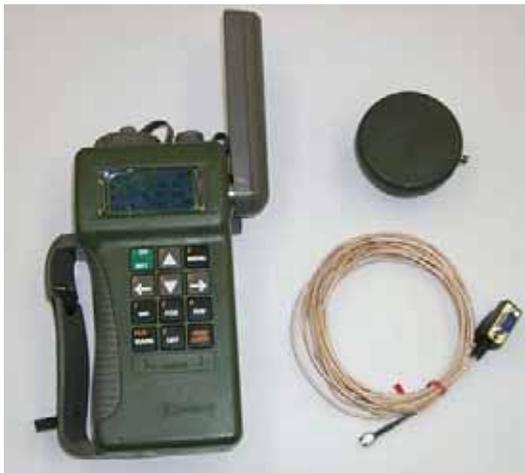
The PLGR+96 FED is a five-channel, single-frequency Precise Positioning System (PPS) P(Y) Code receiver with built-in antenna. It has been evaluated in other MTDC reports and the accuracy of the receiver hasn't changed significantly with S/A turned off. The receiver contains a security module that can eliminate the positional error intentionally introduced when selective availability (SA) was enabled and it decodes the encrypted
