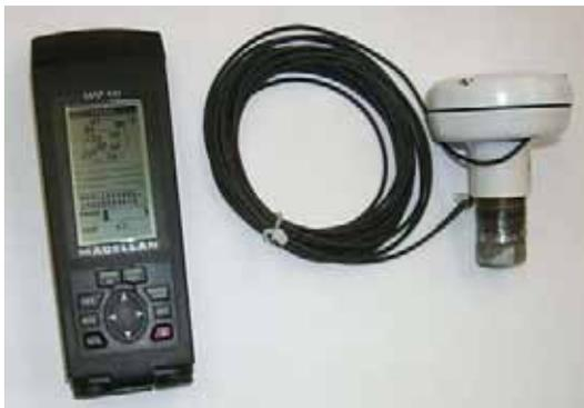
The Magellan Map 410 is a 12 parallel-channel receiver with a detachable signal-sensitive antenna. It has a built-in worldwide background map and detailed basemap for the Americas includes cities, lakes, rivers, railroads, coastlines, interstate, national and state highways. It has a built in altimeter. It can store 500 waypoints and 20 routes with 30 legs. It automatically averages your position
