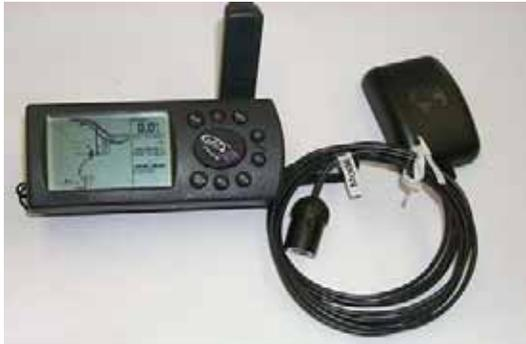
**The Garmin GPS III** is a Differential-ready 12 parallel channel receiver that continuously tracks and uses up to twelve satellites to compute and update a position. It has acquisition Times of, approx. 15 seconds warm and approx. 45 seconds cold. It has a continuous update rate of 1 second. It can store 500 waypoints with symbols and 20 reversible routes, and a track log of 1900 points. It
