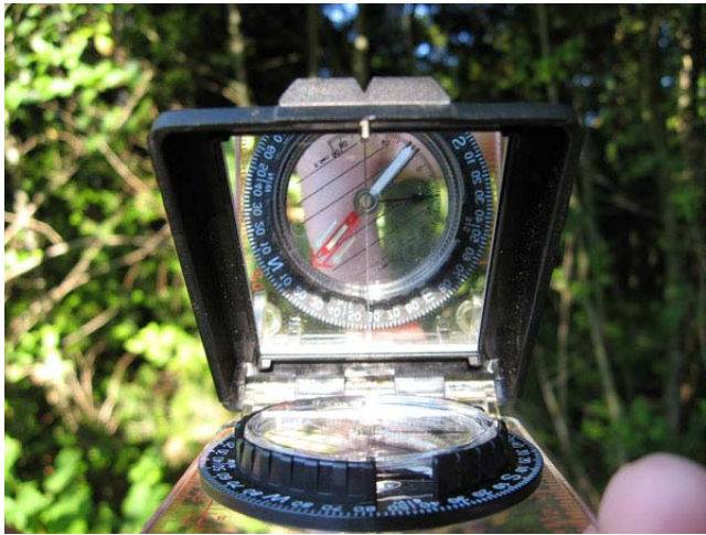
Figure 3-5: If your compass has a mirror, you can use this to watch the needle and make sure it lines up while keeping the compass level. Sight through the notch at the top to see where you need to go.
