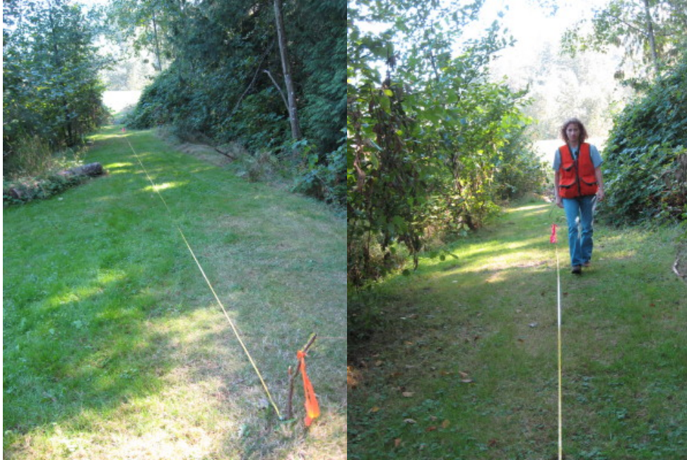
Figure 3-1: Mark out a distance of 1 chain (66 feet) in a flat area such as your lawn or driveway. Walk this distance several times, counting your paces as you go.
