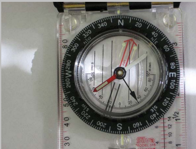
Figure 3-4b: An azimuth compass reads all the way around the compass from 0° to 360°.
