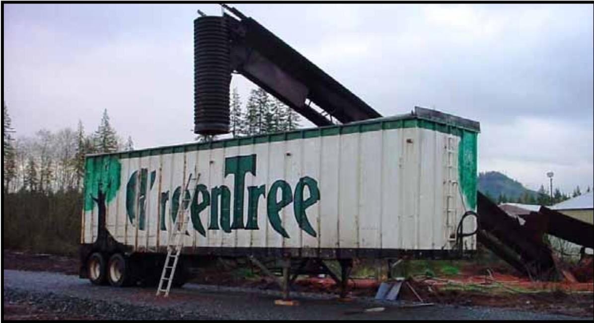
**Figure 15. Chip van receiving shingle waste at Premium Mill in Beaver, WA.**
