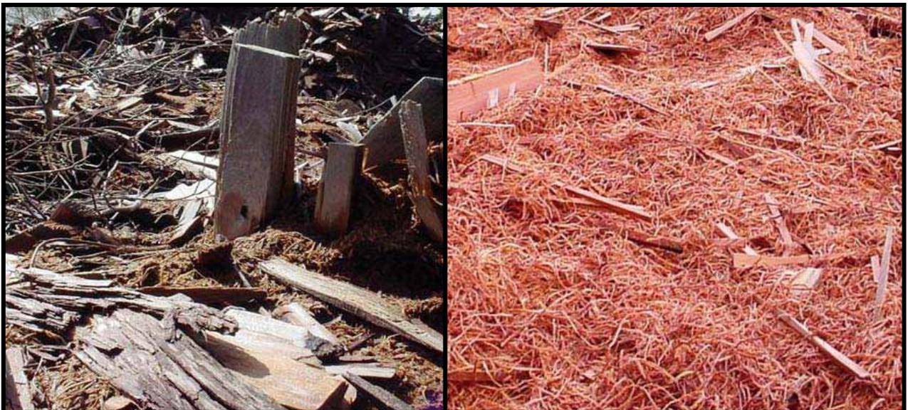
Figure 11. Old waste compared to fresh mill waste. Note the lack of bark and chunks in current material on right.
