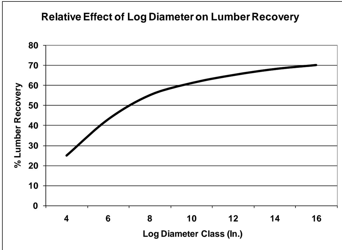
**Figure 3.2.1. The relative effect of log diameter on lumber recovery (Dramm).**
