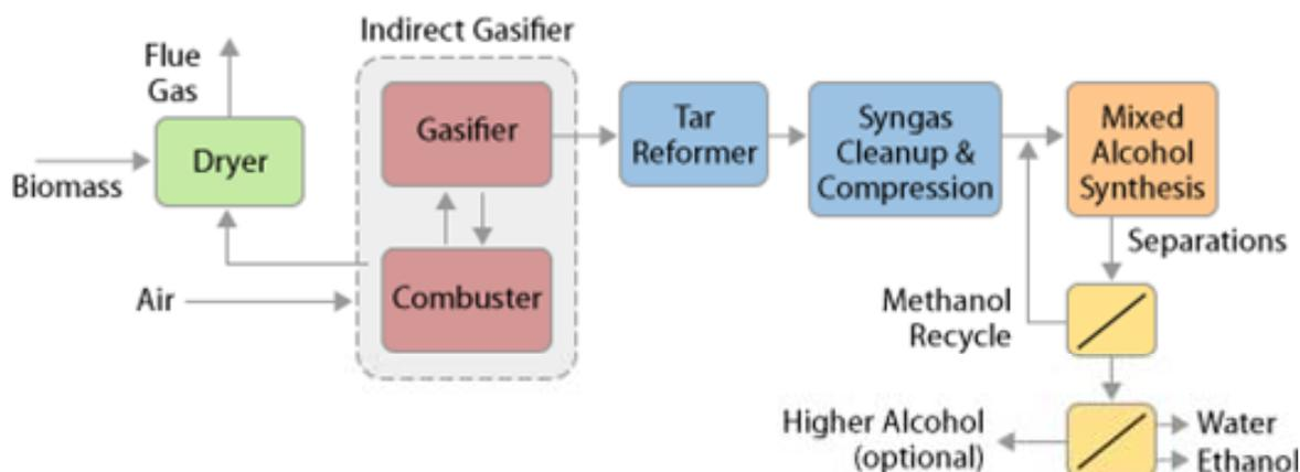
Figure 1.4.10. Schematic for thermochemical conversion of biomass to ethanol (EEREc).
