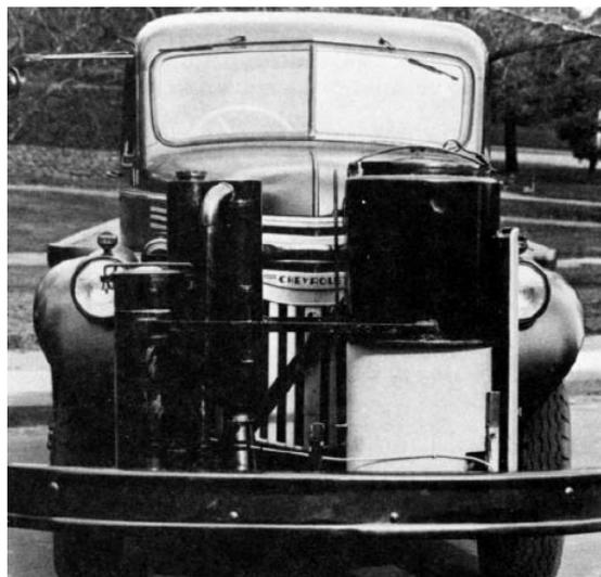
**Figure 1.5.5. Truck equipped to operate with wood chip gasification system (General Motors).**
