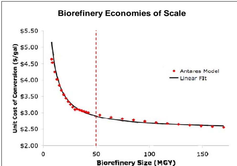
Figure 4.1.7. Biorefinery economies of scale (from WGA 2008b, Antares 2008).
