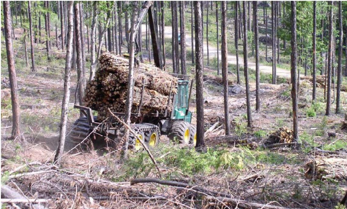
Figure 3.3.7. John Deere 1490D recovering slash bales from forest thinning in OR (McNeil Technologies).
