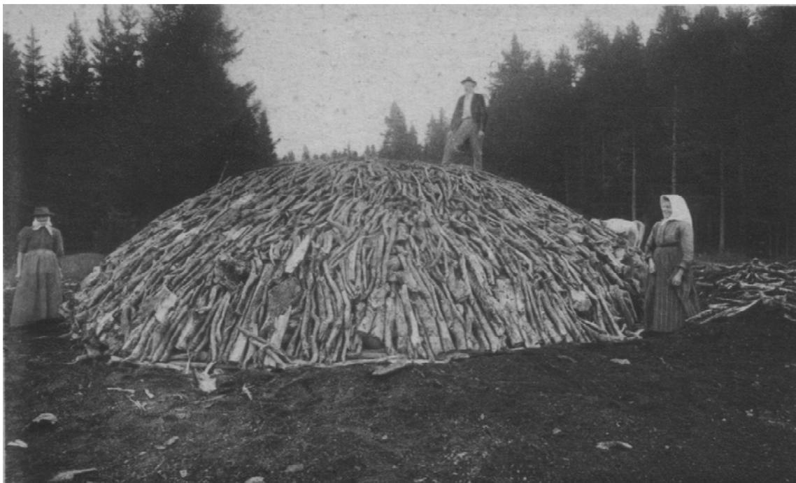
**Figure 1.5.4. Wood pile for charcoal production before being covered with soil and fired around 1890 (Wikipedia).**
