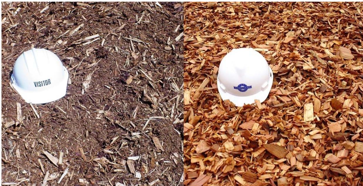
**Figure 1.4.2. Comparison of hog fuel on left and clean wood chips on right (Mason).**
