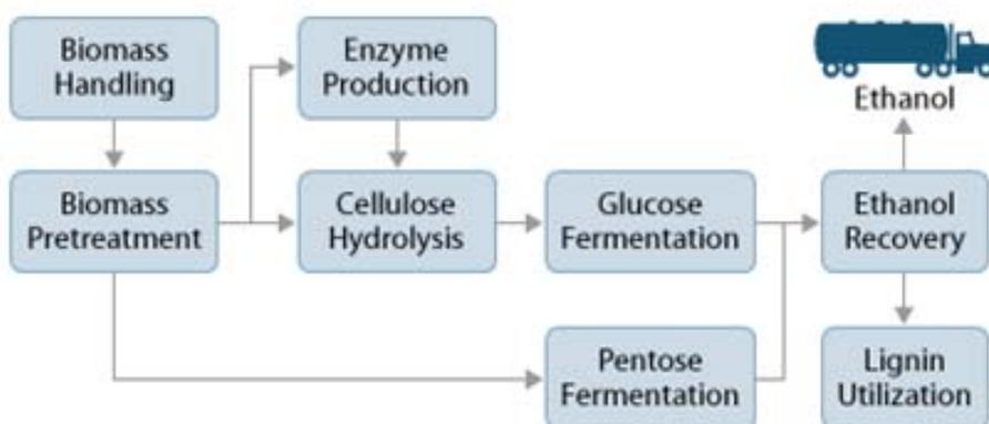
Figure 1.4.9. Schematic for biochemical conversion of biomass to ethanol (EEREc).
