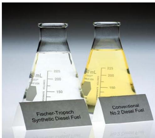
**Figure 1.4.12. FT diesel and fossil diesel (NREL)**
