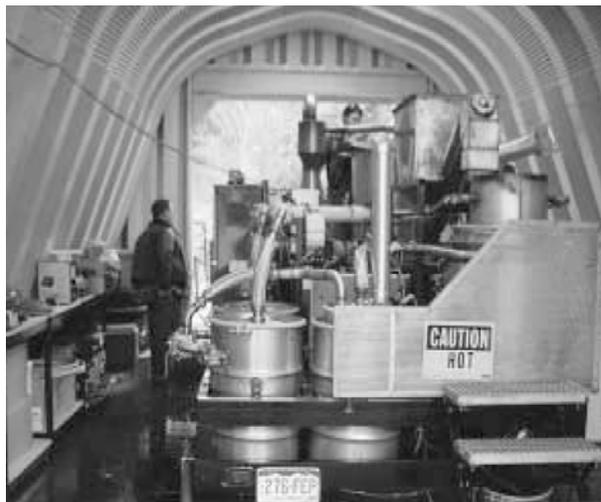
**Figure 1.4.8. Gasification fueled 15 kW generator. Hoopa Indian Reservation (Bain and Overend).**
