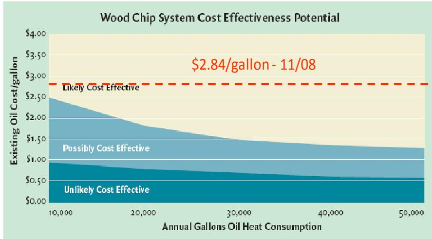
Figure 4.3.2. Wood heating system as compared to 11/08 heating oil price (from Maker 2004 and EIA 2009a).
