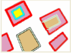
Figure 2 - The red features represent the forested areas. The highlighted cyan features represent parcels and are selected because they are completely within the forested area.
