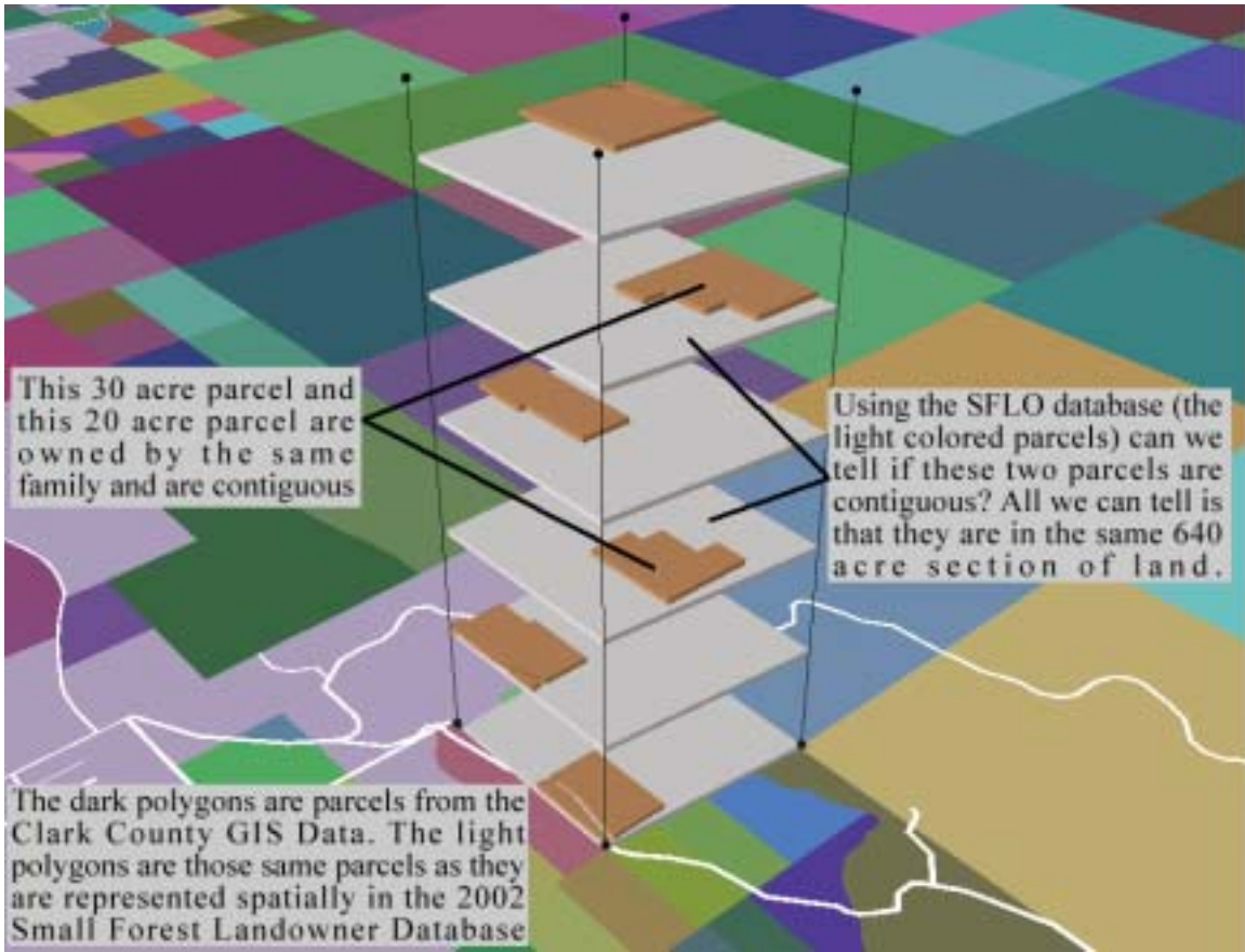
Figure 4 - The difficulty of determining contiguousness using tabular County Assessor data. Each tax parcel in the database is represented by a polygon that is the shape of the 640 acre section of land that the parcel is in.
