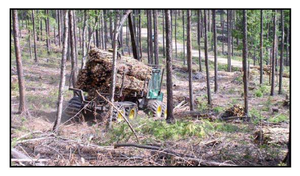
Figure 19. Removing bales of forest biomass during forest thinning activity. Source: McNeil Technologies, Inc.
