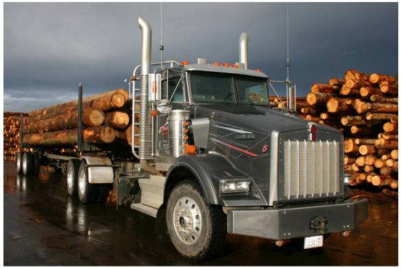
Figure 1.5. Contemporary 5-Axle log truck (Log Trucker Magazine).
