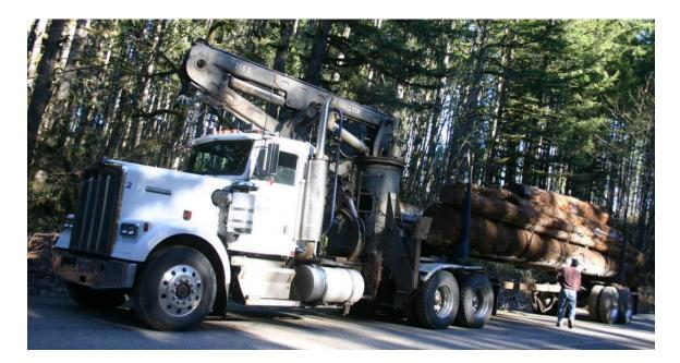
7) 5-Axle Self-Loading Log Truck (Log Trucker Magazine).
